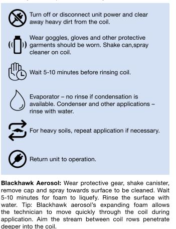
**Condensers:** Spray cleaner into the coil. Blackhawk's expanding foam will penetrate throughout the coil. Wait a few minutes for foam to liquefy and remove grease and grime within coil. Rinse thoroughly. For stubborn or heavy deposits, a repeat application may be necessary.
